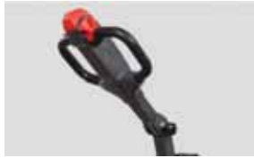
Ayarlanabilir tutma kolu / Adjustable tiller position for ergonomics
